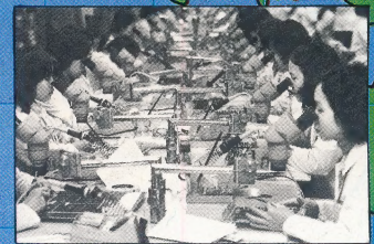
Skilled workers use microscopes to place circuits on a PCB
